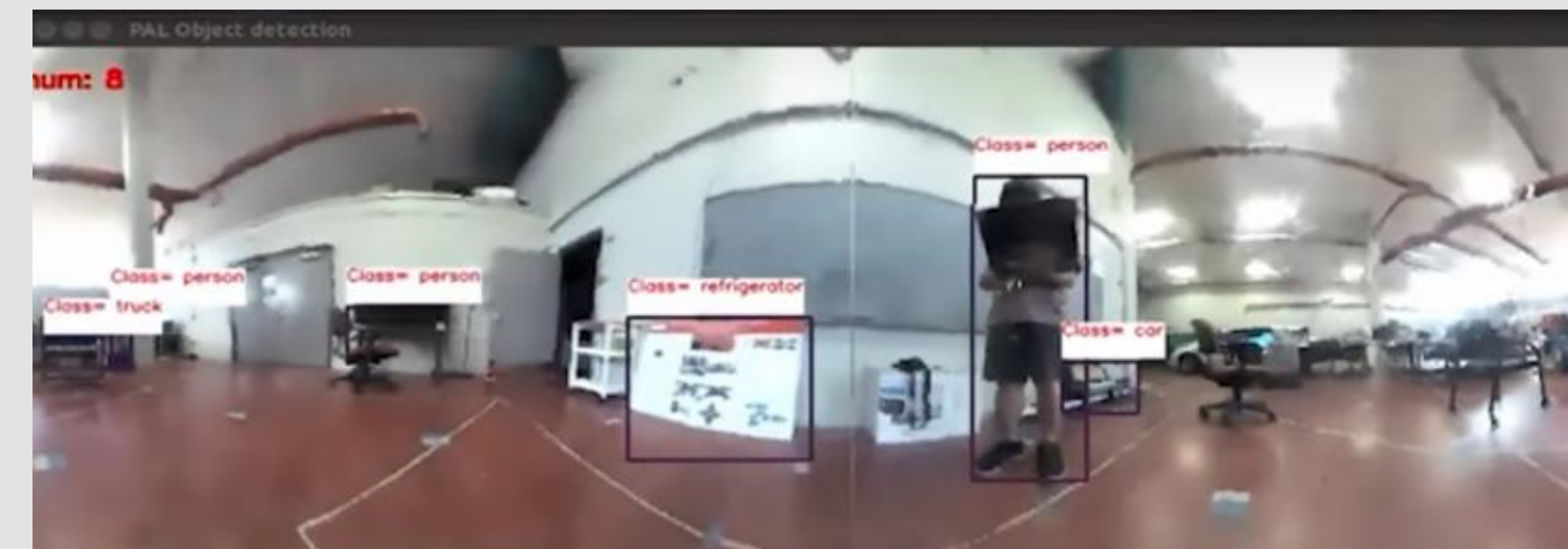
Figure 4: Object Detection by using PAL 360° camera
